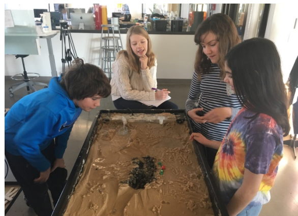
A lab group observes their erosion control system consisting of rip-rap and geotextile
