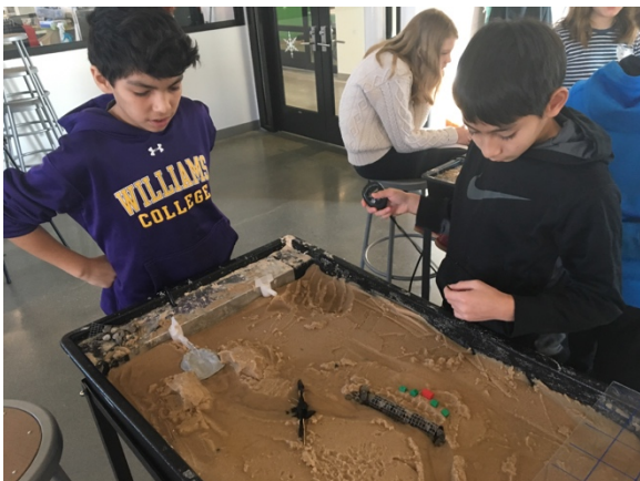
Sixth graders test their erosion control system consisting of Gabion baskets, a check dam, and geotextile
