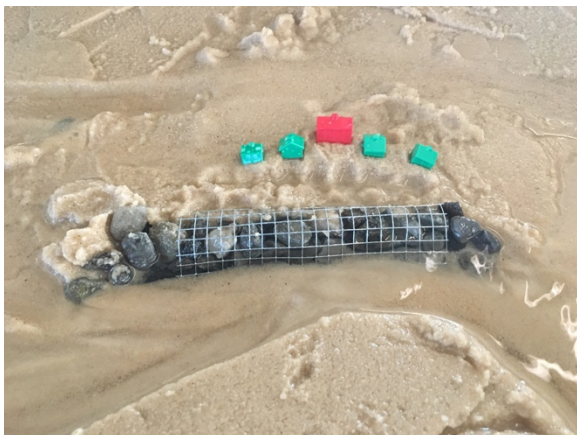
A lab group's erosion control design consisting of Gabion baskets (mesh filled gravel blocks) backed by geotextile
