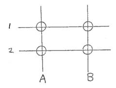
If half the necessary current needed to magnetize a core were applied to wire 1, and if this same amount of current were applied to wire A, the core that is at their intersection would become magnetized. The cores at the intersection of 2 and A, and 1 and B would only get half the necessary current and would not magnetize. This is called coincident current switching. 27
